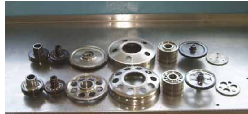
Comparison between original and lightened gears
